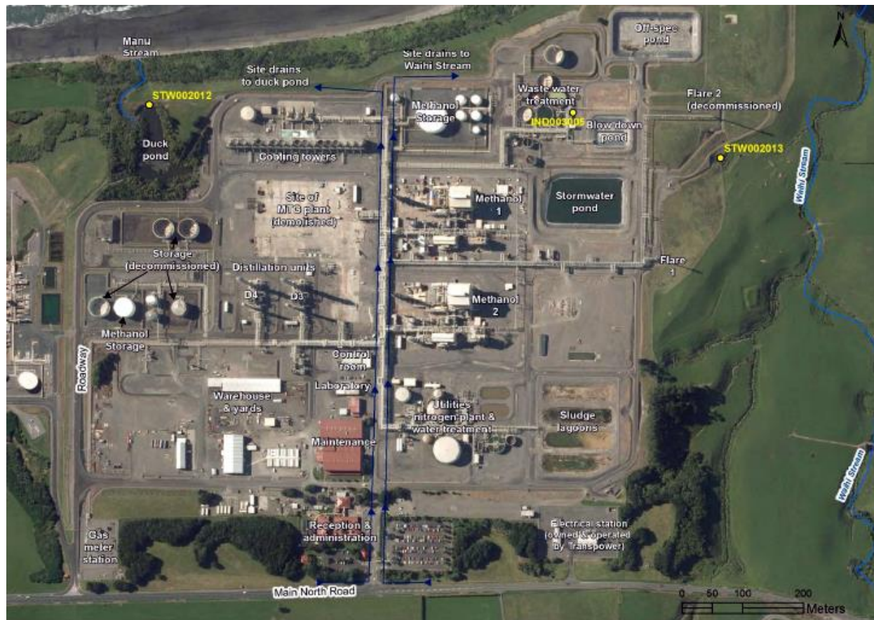
Methanex Motunui site layout with water sampling locations (TRC, Jan 2017)
