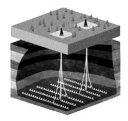
The diagram above has markers on the laterals showing where they will be perforated to allow the fracking fluid access to the targeted rock and after fracking, the perforations will allow oil, gas and contaminated water to flow into the well.
